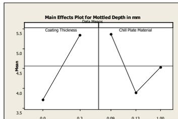
Figure 7. Effect plot for mottled depth in mm.
