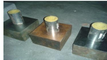
**Figure 4.** Chill plates with mould.
