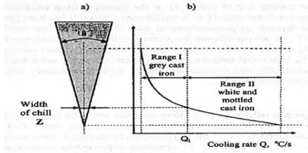
**Figure 1.** (a) Standard wedge-shaped specimen (b) Cooling rate ranges near the tip and along the axial direction of the wedge<sup>2</sup>.
