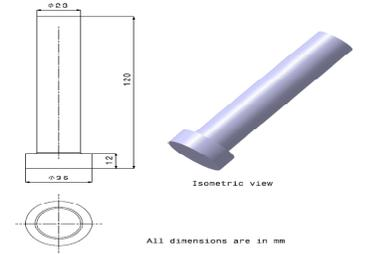
**Figure 3.** Detailed drawing of Cast iron Tappet.
