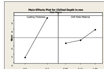
**Figure 5.** Effect plot for chilled depth in mm.
