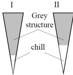
**Figure 2.** Casting for chill and chilling tendency estimation<sup>4</sup>.
