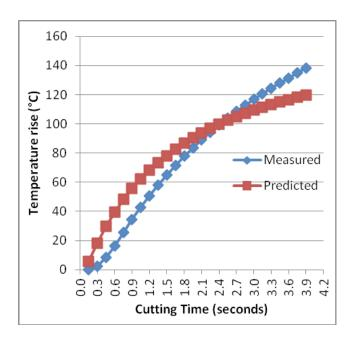
**Figure 3.** Estimated and actual measured temperatures for constant heat influx.
