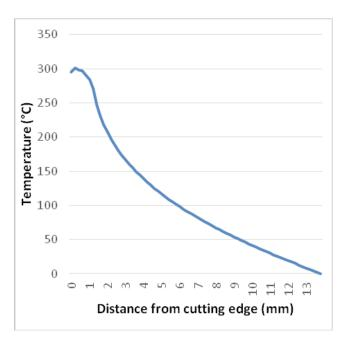
**Figure 5.** Temperature distribution on the tool rake face.
