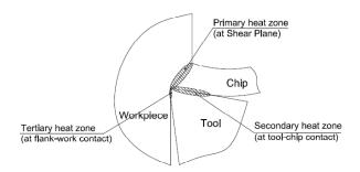
**Figure 1.** Zones of heat generation in machining.
