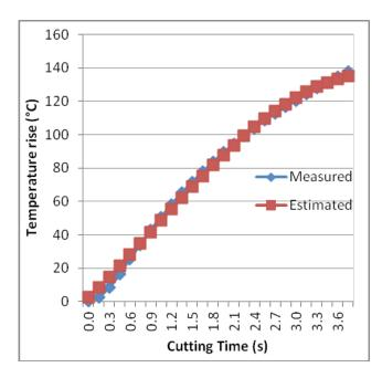
**Figure 4.** Estimated and actual measured temperatures for variable heat influx.
