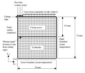
Figure A.1: Geometrical setup for finite difference problem
