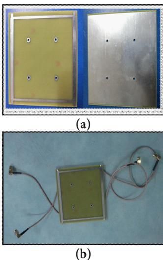
**Figure 32.** (a) Fabricated unequal hybrid coupler. (b) Both conducting and ground plane.
