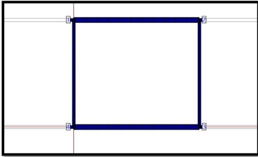
**Figure 20.** Proposed microstrip unequal amplitude quadrature hybrid coupler.
