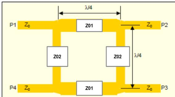
**Figure 2.** Quadrature hybrid built around transmission lines. All arms are  $\lambda/4$  in length.
