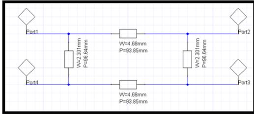
Figure 15. Unequal amplitude quadrature hybrid coupler.
