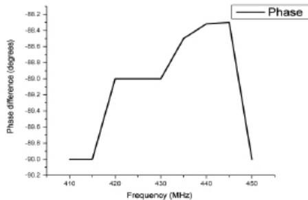
**Figure 35.** Phase difference of the proposed out of phase hybrid coupler.
