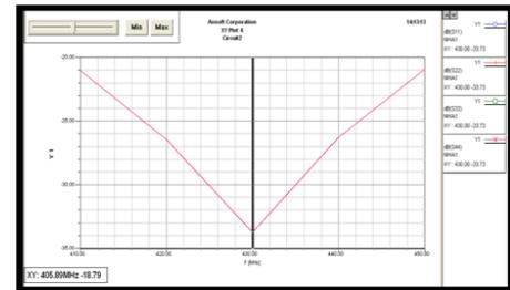
**Figure 7.** Simulated return loss.
