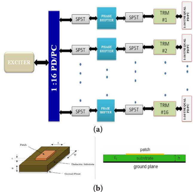
Figure 1. (a) Configuration of t-radar system. (b) Microstrip structure.
