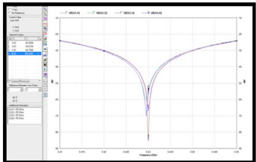
**Figure 23.** Simulated return loss for all ports.
