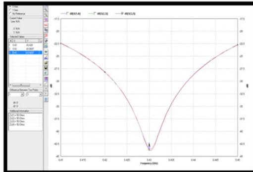
**Figure 25.** Simulated isolation loss for all ports.
