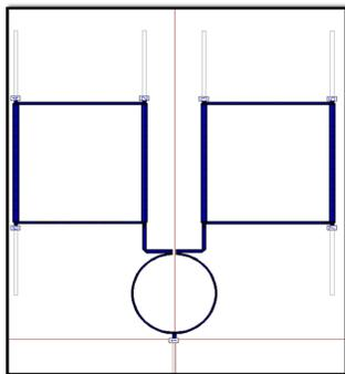
**Figure 27.** 1:4 feeder network.
