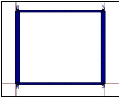
Figure 8. Equal amplitude hybrid coupler.
