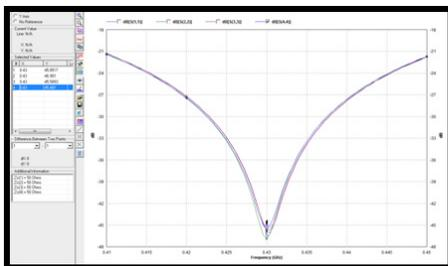
Figure 11. Simulated return loss.
