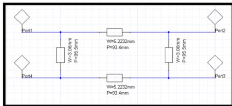
**Figure 3.** Equal amplitude quadrature hybrid coupler.
