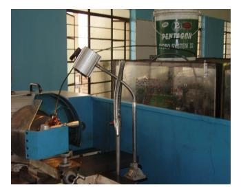
**Figure 8.** MQL setup in conventional lathe.
