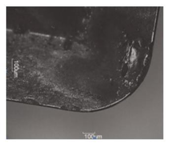
Figure 12. Microscopic image of tool wear in dry machining.
