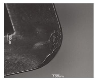
**Figure 11.** Microscopic image of tool wear machined in MQL system.
