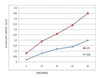
**Figure 14.** Graph showing the difference in auxiliary tool wears.
