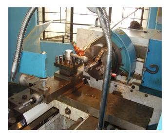
Figure 9. Machining of titanium alloy in MQL setup.
