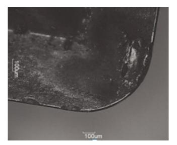
Figure 13. Auxiliary wear observed during machining.
