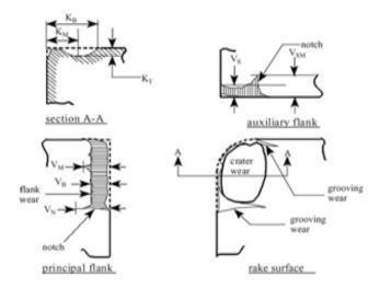
Figure 2. Types of tool wear.
