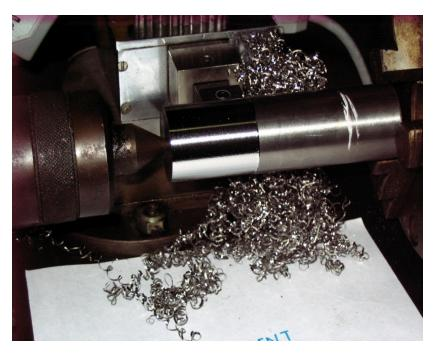
Figure 10. Dry machining of titanium alloy on conventional lathe machine.
