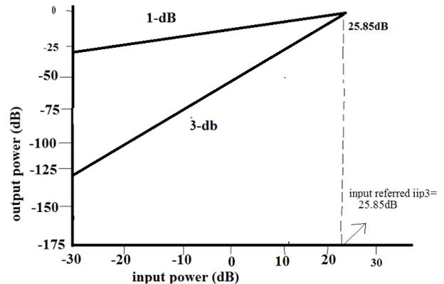
Figure 8. IIP3 measurement of 2<sup>nd</sup> order high-pass filter.
