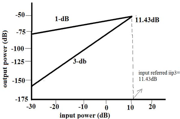
Figure 7. IIP3 measurement of 5<sup>th</sup> order high-pass filter.
