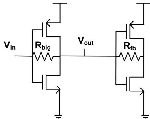
Figure 3. Schematic of a linear voltage amplifier.
