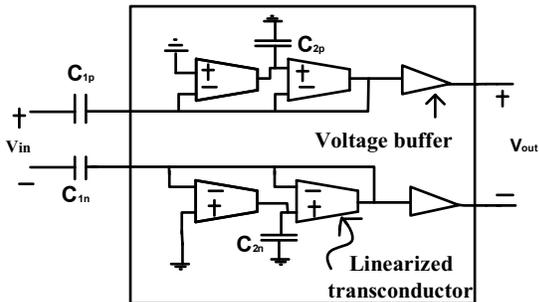
Figure 5. Block diagram of second-order unit high pass filter.
