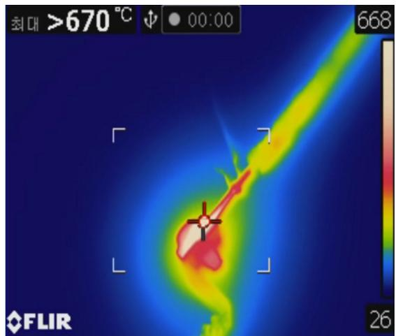
**Figure 4.** Test Results of upper padcontact (0.1mm tightened). (a) Sample. (b) Temperature characteristics (6A). (c) Temperature characteristics (12A). (d) Temperature characteristics (18A). (e) Temperature characteristics (24A).
