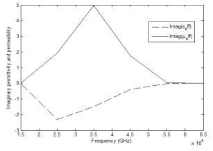
**Figure 5.** Imaginary part of permeability and permittivity vs. frequency.
