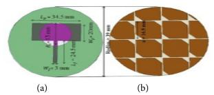
**Figure 6.** Structure of (a) Elliptical slot antenna with microstrip patch feed and (b) Metasurface.
