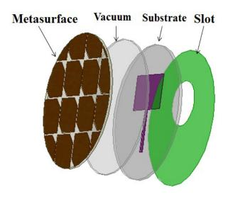
**Figure 8.** Diagrammatic representation of Metasurface antenna.
