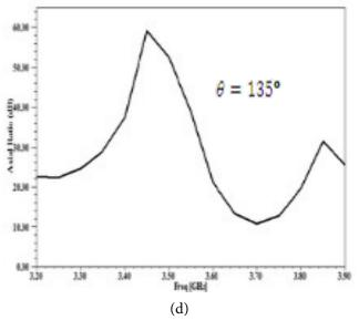
Figure 12. Simulated Axial Ratio for (a)  $\theta = 0^{\circ}$ , (b)  $\theta = 45^{\circ}$ , (c)  $\theta = 90^{\circ}$  and (d)  $\theta = 135^{\circ}$ .
