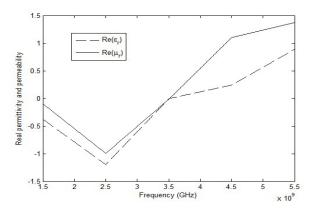
**Figure 4.** Real part of permeability and permittivity vs. frequency.
