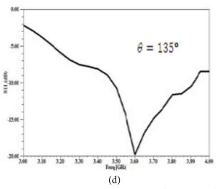
Figure 11. Simulated return loss  $S_{11}$  for(a)  $\theta = 0^{\circ}$ , (b)  $\theta = 45^{\circ}$ , (c)  $\theta = 90^{\circ}$  and (d)  $\theta = 135^{\circ}$ .
