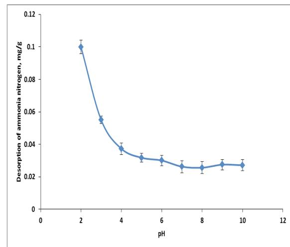
**Figure 5.** Effect of pH on the desorption of ammonia nitrogen from modified empty fruit bunch fibers (Sorption conditions: EFB fibers weight: 15.71 grams, ammonia nitrogen concentration: 50 mg/L, equilibrium time: 40 min and temperature = 27 ± 0.2 °C; desorption conditions: EFB fibers weight: 15.71 grams/L, equilibrium contact time: 40 min and temperature = 27 ± 0.2 °C).
