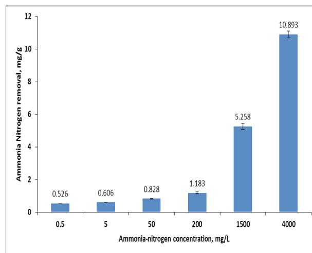
**Figure 1.** Effect of ammonia nitrogen initial concentrations during sorption onto modified EFB (Weight of modified EFB: 15.71 grams, volume of ammonia nitrogen: 1000 mL, contact time: 40 min, room temperature: 27 ± 0.2 °C and pH: 7.0).
