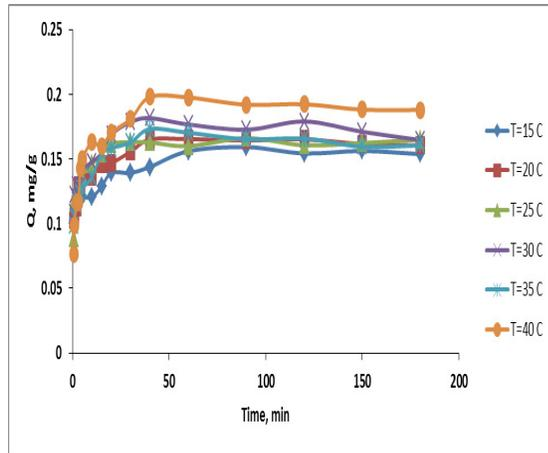
**Figure 2.** Effect of contact time on temperature dependent on sorption capacity of ammonia nitrogen onto the modified empty fruit bunch (Weight of modified EFB: 15.71 grams, ammonia nitrogen concentration: 50 mg/L, and pH: 7.0).
