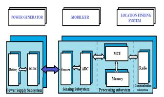
Figure 4. Power system of sensor node in WSN.
