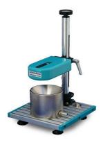
Figure 1. Typical Sketch of Shrinkage-Cone.
