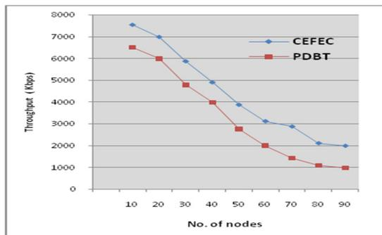
Figure 8. Through put comparison of PDBT and CEFEC.
