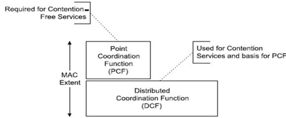
Figure 3. Distributed Coordination Function<sup>18</sup>
