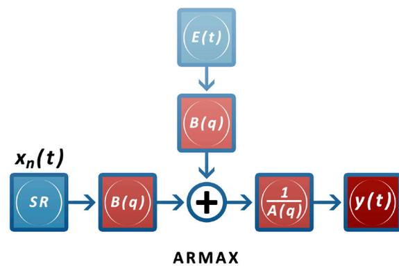
Figure 1. ARMAX model implemented.
