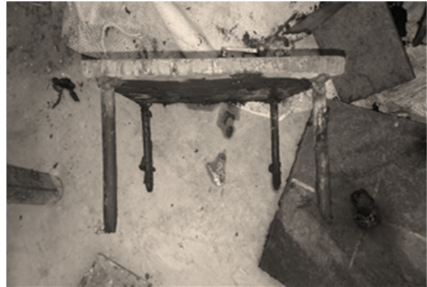
Figure 2. Model rigid pile raft system of 4 piles.
