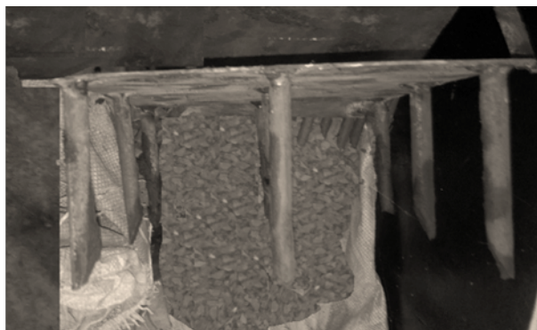
Figure 1. Model flexible pile raft system of 9 piles.
